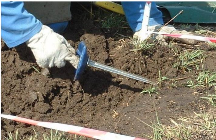
Insert the Pick-prod and twist the blade to break up the ground.
